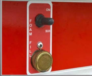
The auto fill feature allows the firefighter to fill the foam cell without having the foam container leave the ground.
