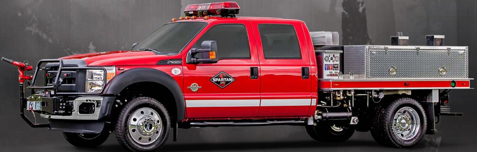
Componentry located under the flatbed deck results in a low profile and low center of gravity for superior off road handling.
